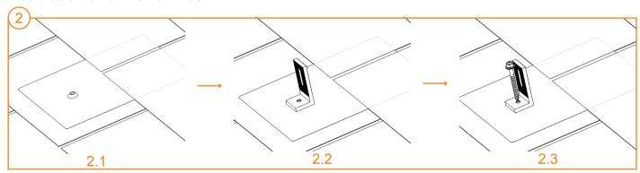
Remove the tile where you are installing the 19# hook by gently pulling and pushing the tile. Place the 19# hook on top of the rafter where it will be installed, then fasten it with three wooden screws M8\*90, finally return the tile to its original position.
