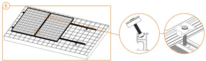
Insert mid clamp nut by tilting it into the top opening of rail, then put the second panel onto rails. Fasten mid clamps with inner hex bolts M8 at all locations where two panels meet. The two SS304 rivets inlaid in the grounding mid clamp have grounding function when fastened tight.
