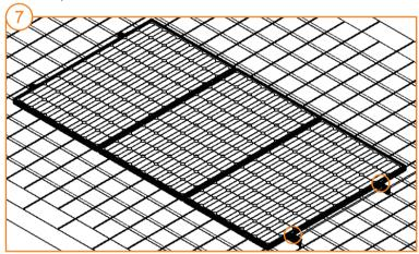
Install all the panels and fasten end clamps at the end of each array. The SS304 rivet inlaid in the grounding end clamp has grounding function when fastened tight.
