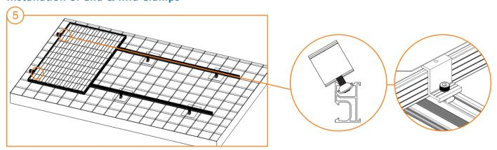
Tilt end clamp nut into the top opening of rail. Put the first PV module on two parallel rails, then fasten the end clamp bolt (inner hex bolt M8) to secure one side of the panel. The SS304 rivet inlaid in the grounding end clamp has grounding function when fastened tight.
