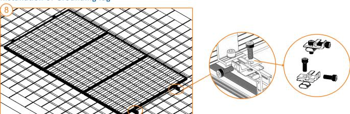
Install a grounding lug (50mm from the rail end) onto each rail line edge with an inner hex bolt M8\*25 and a stainless steel nut, then cross 8.4mm² (greater than or equal to 8AWG) copper wire through all the grounding lugs (fixed by M8\*20 inner hex bolt), finally connect copper wire to the ground. The grounding lug has grounding function when fastened tight to connect rail and copper wire.
